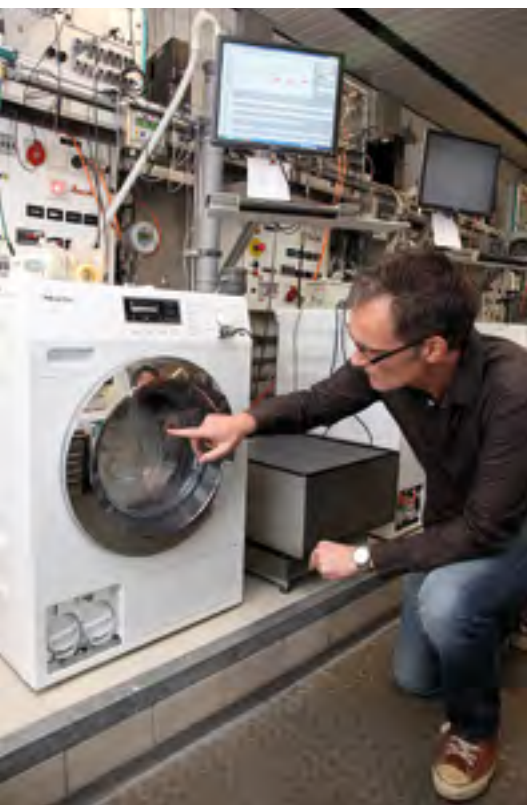
Dirk Sieding explains PowerWash in the laboratory. The flow pump is situated behind the left sealing cap (bottom left picture).
