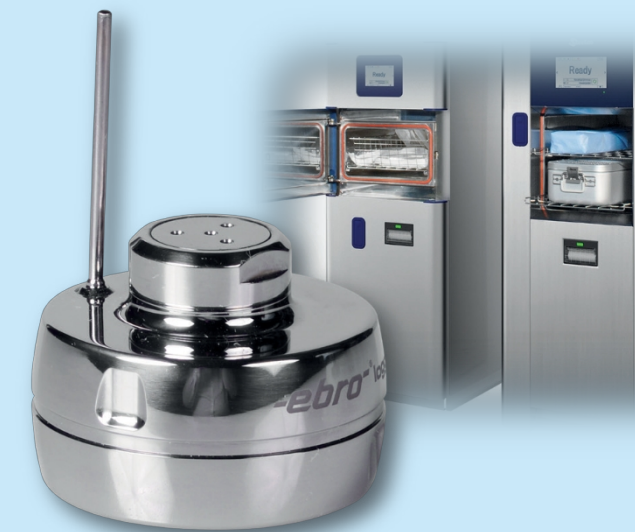
Fig. 1: Independent testing using the EBI 12-TP290 pressure-temperature data logger in the VH2O2 process.
