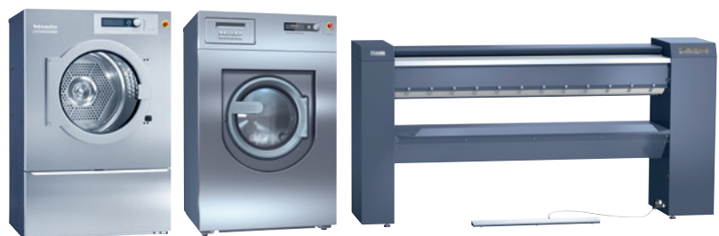
Example of a high-performance in-house laundry: Washing machine and tumble dryer, each with a 20 kg load capacity, cycle time of approx. 70 mins. incl. drying, flatwork ironer with a throughput of 60 kg/h
