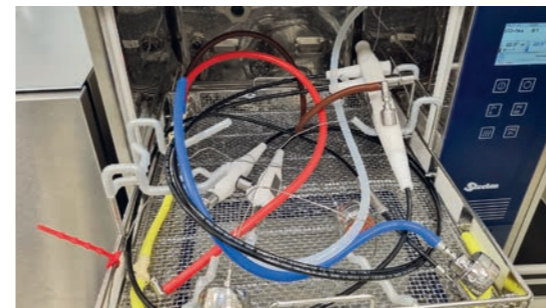
Fig. 3: Spypach „Classic“ endoscope dummy with EB12 data logger for measuring pressures and temperatures in the simulated endoscope.
