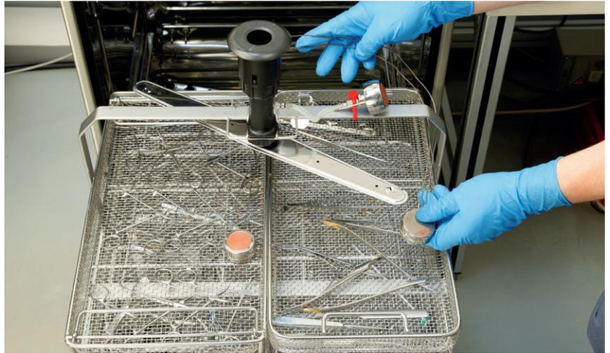
**Fig. 2: Pressure measurement during washer-disinfector process validation.**
