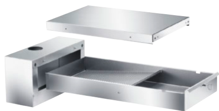
APCL 021 Fluff filter drawer, stainless steel, removes fluff and coarser particles from suds. • For installation on a suitable plinth • Removable for quick and easy cleaning. • Easily removable fluff filter in stainless steel • Volume 24 litres • Diameter of rear connector 70 mm • H/W/D: 25.00 cm – 49.85 cm – 86.00 cm
