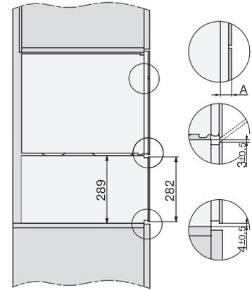
side view, DG, DGM, ESW7x20 installation drawings
