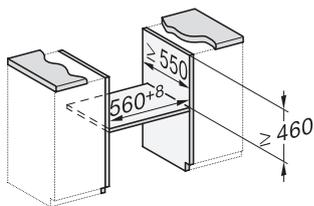
built-in H7000 M build-under, installation drawing
