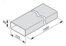
DFK-R1000, Flat-type ducting, 1000 mm, installation drawing
