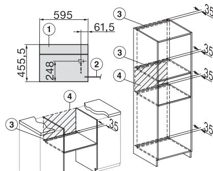
DGC7x40 connections and ventilation 45cm, installation drawing
