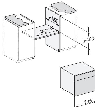
Installation\_DG\_DGM\_DGC\_XL\_ESW7x10\_EVS7010, installation drawings
