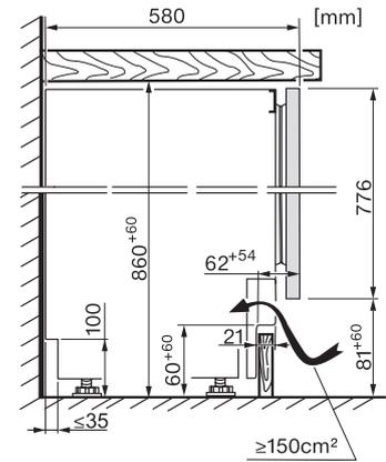
KWTUS7196E, Built-under, side view (installation drawings)
