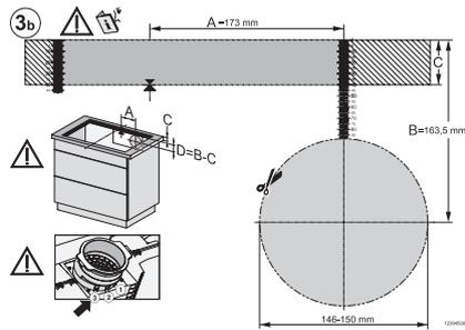
KMDA7676FL-U, KMDA7876FL-U – flush installation, drilling template, Installation depth 21 cm, Installation drawing
