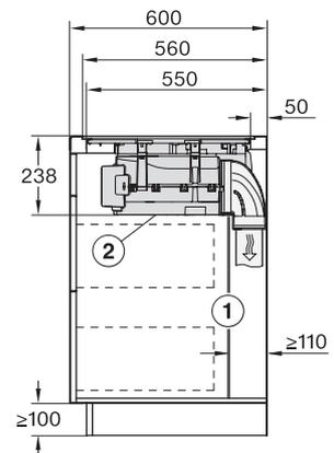
KMDA7676FL, KMDA7876FL – Side view flush – Installation drawing
