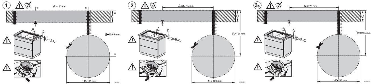
KMDA7676FL-U BlackPerfection, KMDA7876FL-U – flush installation, drilling template, Installation depth 20 cm
