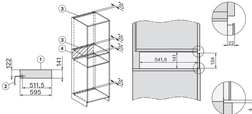
Installation ESW7x10, installation drawing, AU, GB
