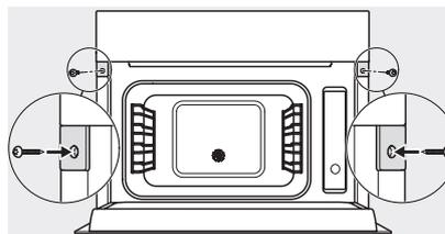
Screw joint DG DGM, installation drawing
