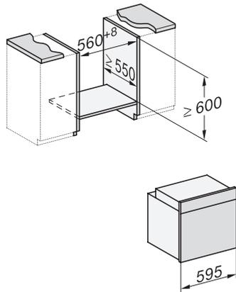
H226x-1B/BP/E/EP/I/IP, H2x6xB/BP, H7x6xB/BP/BPX, H2x6xB, installation drawings
