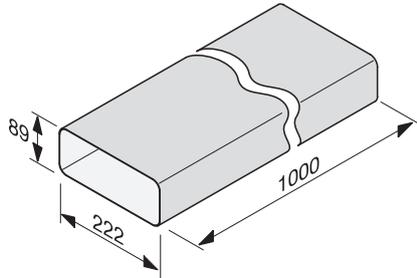
DFK-R1000, Flat-type ducting, 1000 mm, installation drawing
