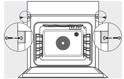
screw joint DGC XXL, installation drawing
