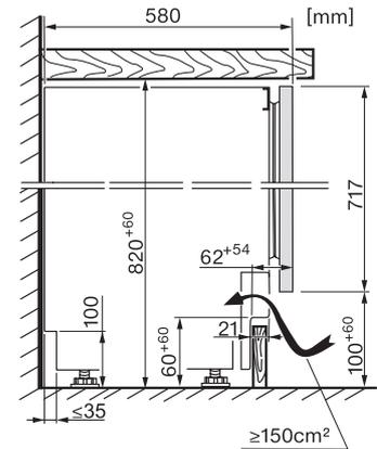
KWTUS7096E, Built-under, side view (installation drawings)
