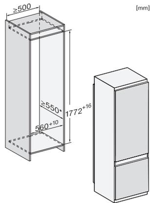
KF7731E, KF7731D, built-in (footnote\*) (installation drawings)
