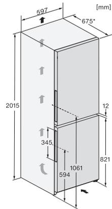
KFN4395DD, KFN4395CD, KFN4397CD, installation sketch (footnote\*) (installation drawings)
