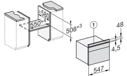
di6465ch DGC7x40-55 built-in build-under, installation drawing, CH
