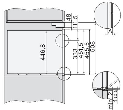
side view DGC 7x40-55 compensating cover at the top, installation drawings, CH
