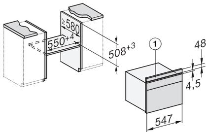
di6465ch DGC7x40-55 built-in build-under, installation drawing, CH
