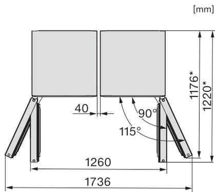
KS4887DD, FNS4882D, top view, Side-by-Side (\*footnote) (installation drawings)
