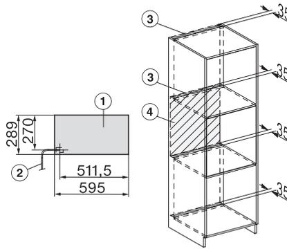
ESW7x20, DGM7x4x installation drawings
