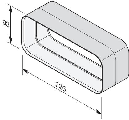
DFK-V, connecting plate, flat-type ducting, installation drawing
