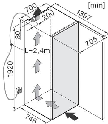
KWT6831SG, KWT6832SGS, KWT6833SG, KWT6834SGS (Installation drawings)
