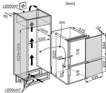
KF35532-55ED, KF35532-55ED-1 (installation drawings)
