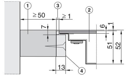
KM 6367 PowerFlex (Installation drawing) – Installation in granite or marble worktops
