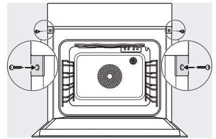
screw joint DGC XXL, installation drawing
