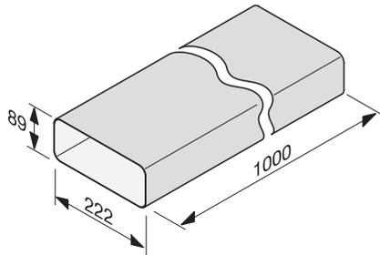
DFK-R1000, Flat-type ducting, 1000 mm, installation drawing
