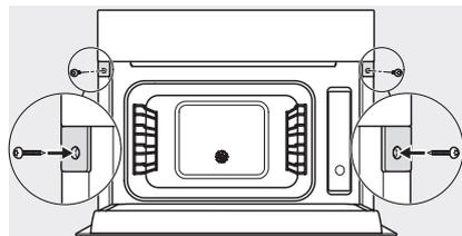
Screw joint DG DGM, installation drawing
