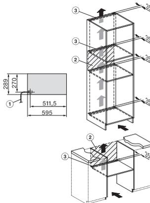
built-in ESW7x20, installation drawing
