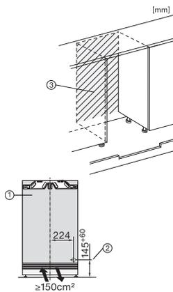
KU7016D, KU7015D, KU7035D, KU7135D, FNUS7140C, Built-under, installation drawing (\*footnote) (installation drawings)
