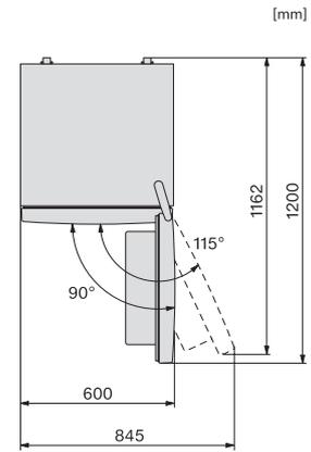
KF4372CD, KF4392CD, KD4050E Active, KD4052E Active, KD4072E Active, KD4172E Active, top view (installation drawings)
