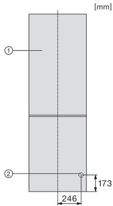
KF4372CD, connection sketch (footnote\*) (installation drawings)
