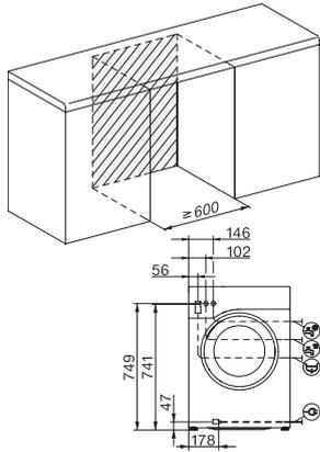
W1 drawing, facia 5 degree, mesures in mm
