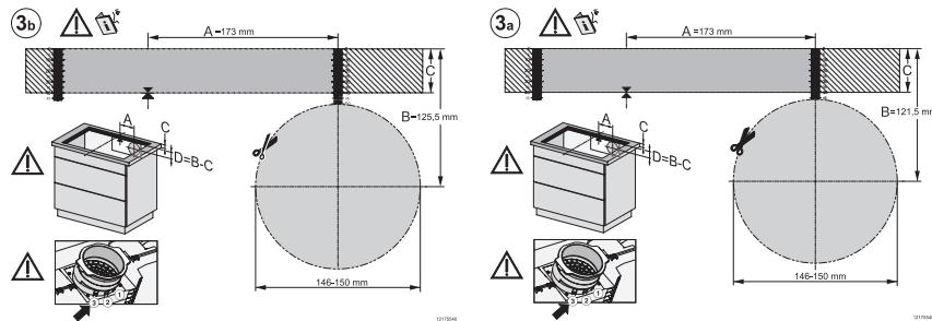
KMDA7272FL, KMDA7473FL – flush installation, drilling template, Installation depth 21 cm, Installation drawing
