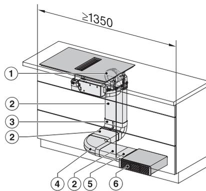
KMDA7676FL, KMDA7876FL – Installation variant 4 Circulating air-drawing
