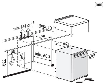
K4003D ws, K4002D ws, installation sketch (\*footnote) (installation drawings)
