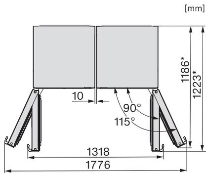
KS4783ED, FNS4782E, top view, Side-by-Side (\*footnote) (installation drawings)
