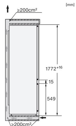
KF7742B, KF7742C, KF7742D, KF7772B, side view
