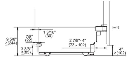
KF2901Vi/SF, KF2911Vi/SF, KF2801Vi/SF, KF2811Vi/SF, KF2981Vi/SF, sideview, MasterCool, installation drawings
