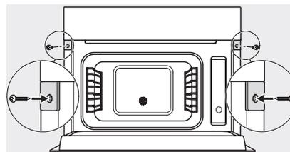
Screw joint DG DGM, installation drawing
