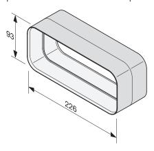
DFK-V, connecting plate, flat-type ducting, installation drawing
