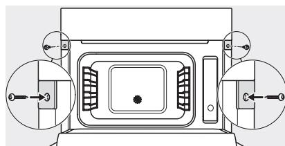
Screw joint DG DGM, installation drawing
