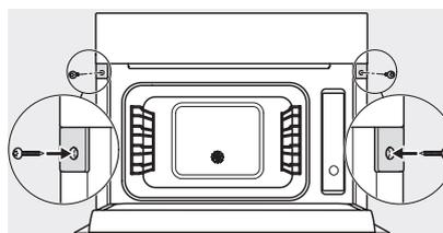
Screw joint DG DGM, installation drawing
