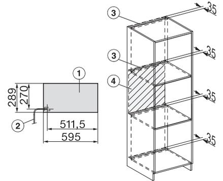
Installation DG, DGM, DGC XL, ESW7x20 installation drawings
