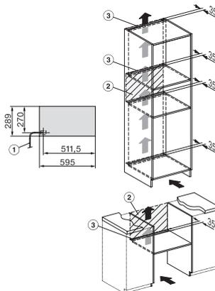
built-in ESW7x20, installation drawing
