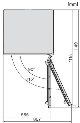
KU7016D, KU7015D, KU7035D, KU7135C, FNUS7040D, FNUS7140C, Built-under, top view (installation drawings)
