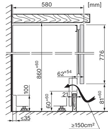
KWTUS7196E, Built-under, side view (installation drawings)
