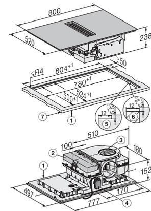
KMDA7676FL-U, KMDA7876FL-U – flush installation, drilling template, Installation depth 24,8 cm, Installation drawing
