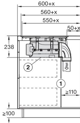
KMDA7676FL, KMDA7876FL – Side view flush+X – Installation drawing
