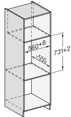
ESW7x10, EVS7010, DGC7x6xHCPro, DGC7x6xHCXPro installation drawings
