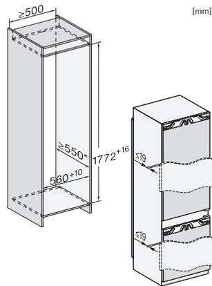
KF7742D, KF7772B, built-in (footnote\*) (installation drawings)
